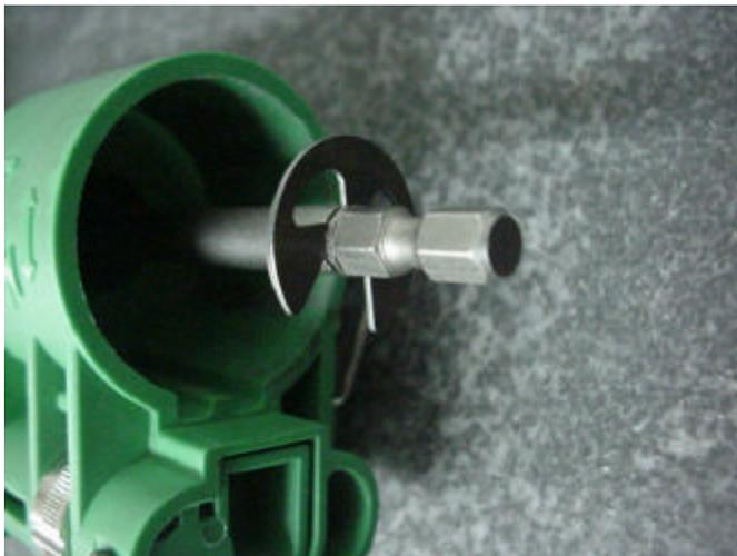
**The Bit-Retaining clip is important as it prevents the hex bit from accidentally hitting the feed latch, as well as reducing problems if the bit happens to stick to a screw. Please insure that it always installed on the Hex bit before use. The adaptor assembly is only used with the Square and Phillips bits.**
